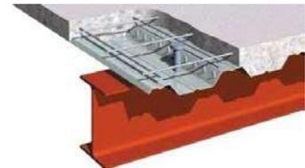
The structural steel system will consist of 127 mm reinforced concrete topping on steel deck supported by composite steel beams (with shear studs) and steel deck. The columns will also be steel wide flange sections. The steel members would require fire proofing, but the topping on the deck can be designed to meet the fire separation requirements by increasing the topping thickness and avoiding spraying the underside of the deck.
