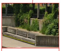
LED RGBW Strip light to be Install under the seating area. Power and data to be supplied from gazebo feed.
